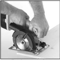
Fig 9. Proper Holding Grip.
